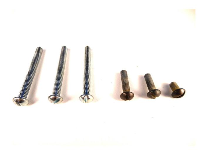
To cut the screw to the proper length, I use a Dremel tool with an Emery cutting wheel attached (see picture). While holding the screw with a pliers, I cut the screw straight across at the proper length. Then I bevel the cut edge of the screw by holding it at an angle against the side of the cutting wheel and rotating the screw (I do this by hand). This will make it easier to get the screw started into the threads of the hole.
