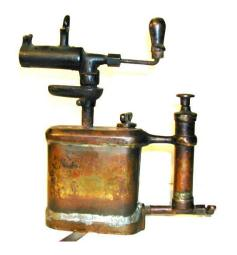
On the Baum & Bender auto torch to the left, you can see that there was a significant amount of solder around the base of the tank. After removing the bulk of the solder, the key was to make the solder line look correct when finished. I used steel wool to clean off any remaining excess solder. This allowed me to make a more
