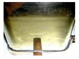
Even after you have removed the excess solder, the areas that were incorrectly covered with solder will still appear white in color. To return them to the brass or bronze color, use a 400 grit wet/dry metal sandpaper. The layer of solder is very thin and sands off with ease. After buffing, the scratches from the steel wool and sandpaper
