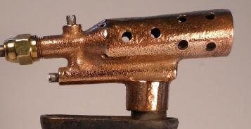
The photos above and left are of a C&L model 47 with minor variations from the torch above. On this torch, the lower pump support is threaded on the outside. This torch also has the C&L shield stamped on the front of the tank.
