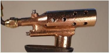
The photos above and left are of a Clayton and Lambert model 47. This torch has the lower pump support threaded on the inside.
