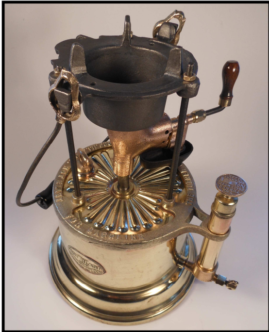
A Turner/White No. 31 one-gallon brass-tank "Combination" Furnace. From the collection of Graham Stubbs , see details on page 15.
