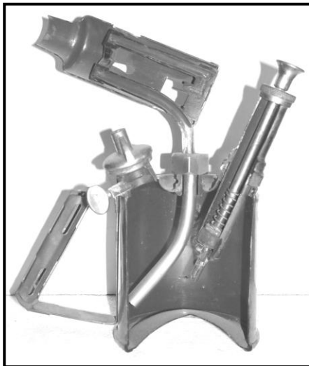
SAMUEL HEATH & SONS (UK) ONE-PINT BLOWLAMP CUTAWAY SAMPLE (Photo Bob Prichard)
