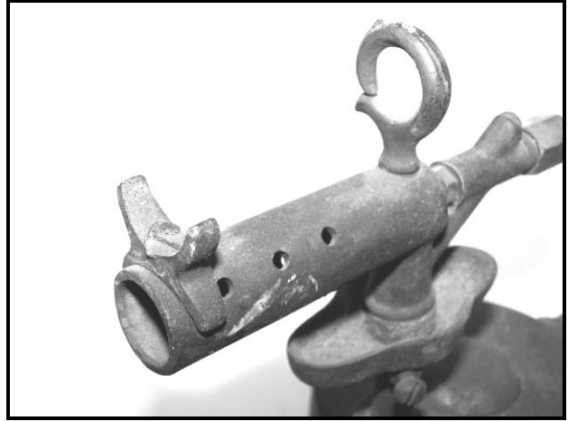
WHITE MFG. NO. 54 TORCH BURNER WITH SOLDERING IRON HOLDER (Photo Charles Smith)
