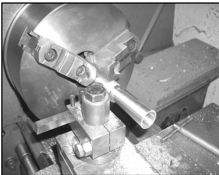
The burner nozzle being tapered. One end has already been threaded.
