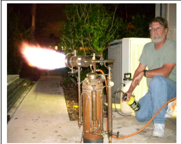
Mike Gratz firing up ENORME CHALUMEAU. Note the orange fuel line feeding propane to the burner assembly.
