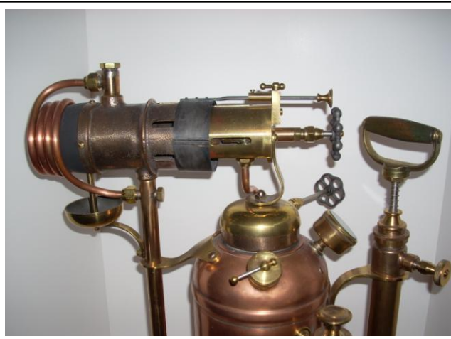
Burner details for ENORME CHALUMEAU. Most all of the components are fabricated from raw stock or are spare parts.
