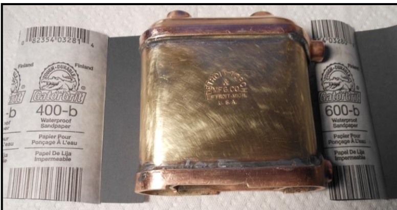
Fuel tank partially completed using various sandpaper grits.
