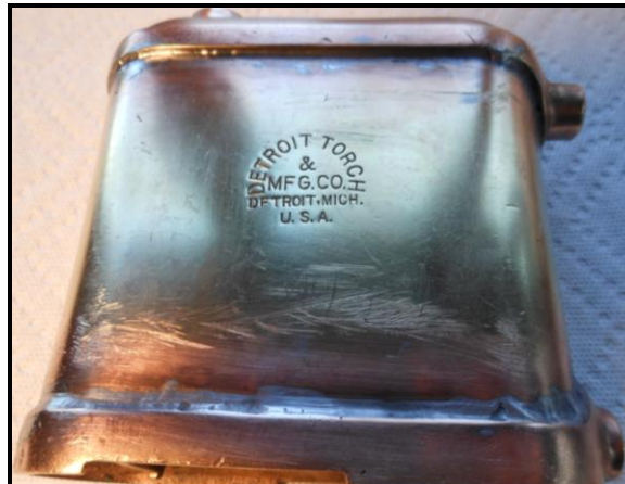
Fuel tank with excessive scratches
