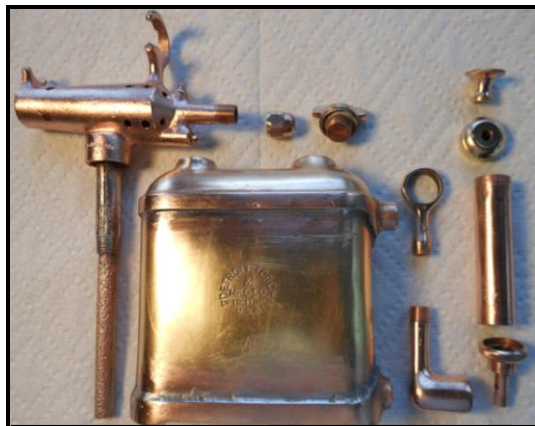
Detroit Auto torch after cleaning
