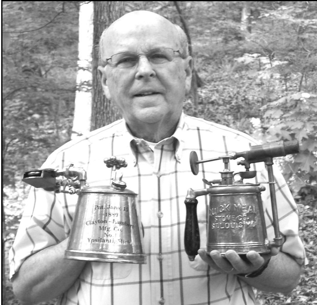
Charles is holding a circa 1889 Clayton & Lambert "The Boss" Paint Burner in his right hand and a circa 1893 Quick Meal Stove Co. Paint Burner (recently acquired from member Mark Pedersen) in his left hand.
