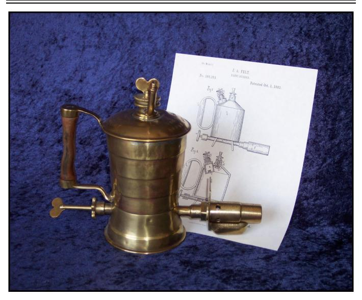
Shown is an "ACME" Paint Burner made by the W. P. Pope Co. of Brooklyn, NY. The "ACME" design is based on a US patent issued to John A. Felt of Kent, OH on October 3, 1882, and as seen in the background.
