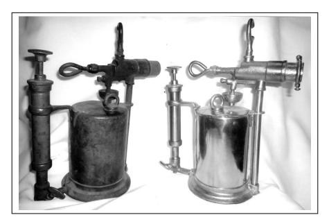
On the left in this photograph is the Quick Meal torch before restoration, missing the SI rest that can be seen in the previously restored torch on the right.
