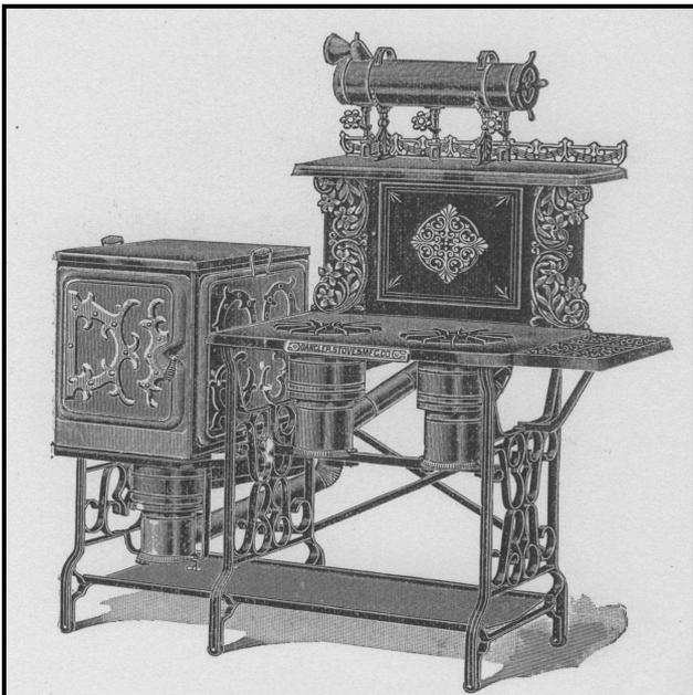
The vapor stove shown in the illustration at left is a No. 242 Process Stove with two burners and an oven that sold for \$22 in 1898. The burner assemblies are the cylindrical tubes located under the burner plates and oven. The gasoline fuel tank is the long tube affixed to the top of the stove.
