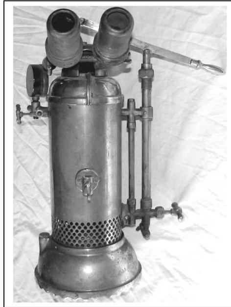
Weighing in at thirty-one pounds and standing eighteen inches tall, this is a very impressive tool. The construction is primarily of nickel-plated steel.
