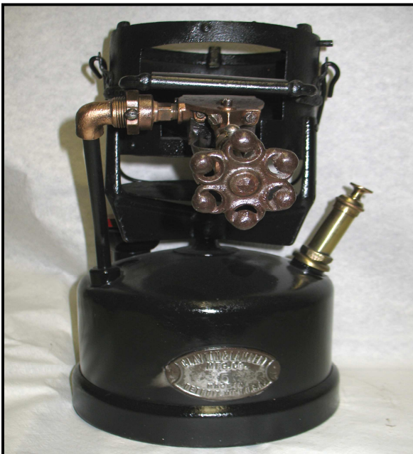
Clayton & Lambert No. 5 Firepot with steel fuel tank. Photo by Dave Kolb, see page 4.
