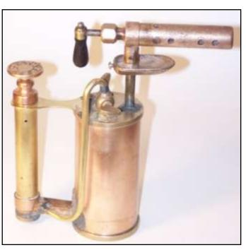
The cast burner tube  $\uparrow \uparrow \uparrow \uparrow$  has four internal "ribs" or "struts" running parallel to its length, a feature that has not been seen before. The pump knob is cast with "PAT APP FOR", and after checking our patents, we could not identify the torch. Perhaps one of our members has a similar torch....especially with the "ribs" inside the burner tube. Please contact us if you have such an unusual torch in your collection.
