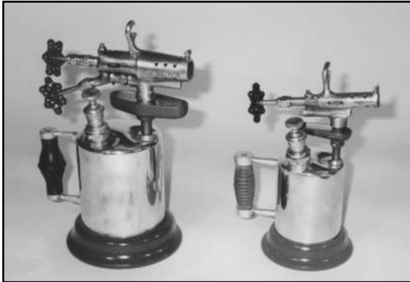
Two Clayton & Lambert Blow Torches with the Patented "Cushion Band" feature. Photo by Dick Sarpolus
