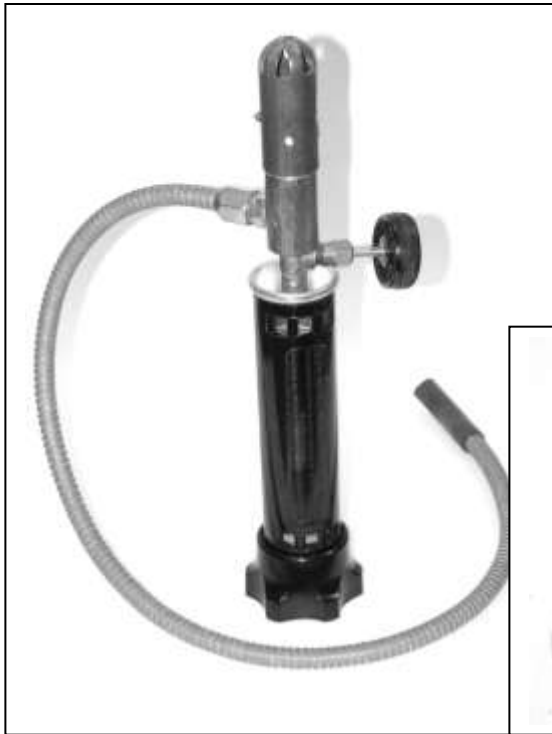
Frigidaire Refrigerant Detector Adapted From a Justrite Torch
