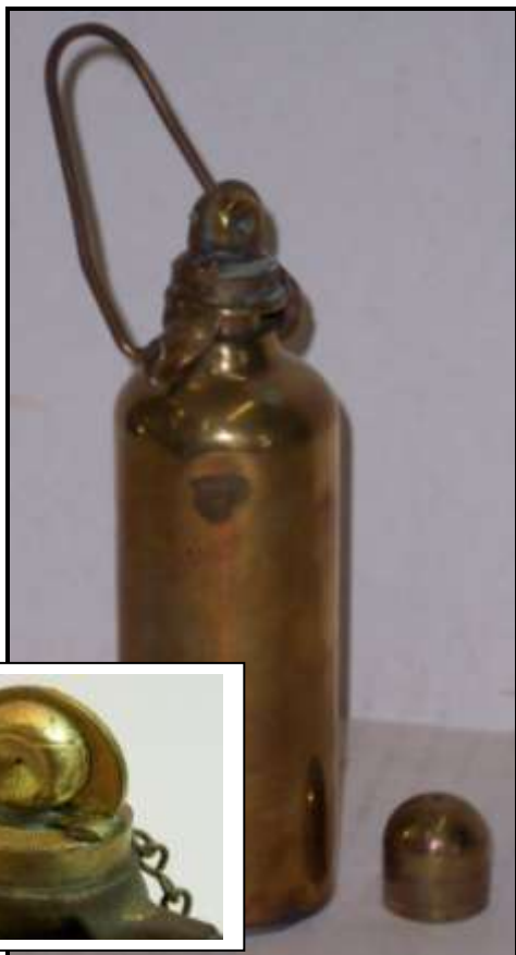
SODERALL Self-Acting Blow Torch Photo by Ron Carr
