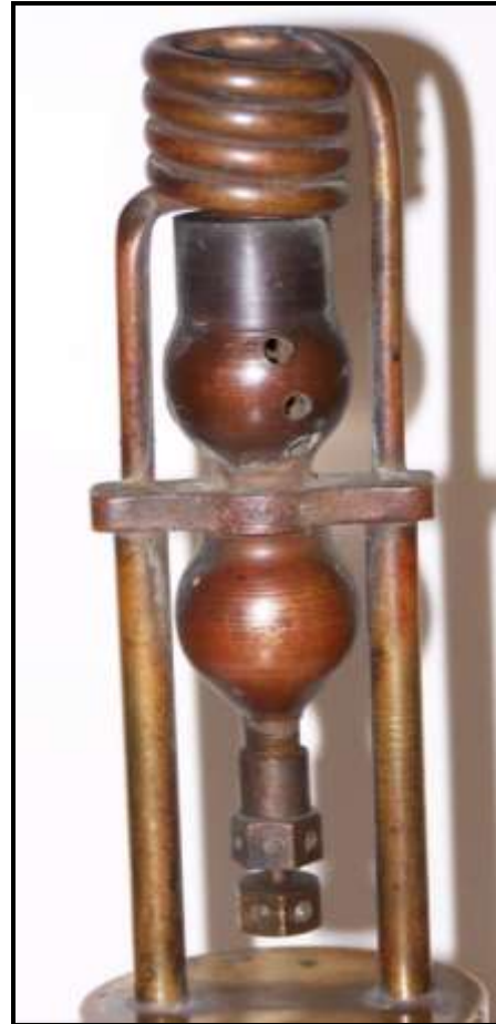
Frank J. Mann SHSI Details of burner head less soldering iron tip Photo by Charles Smith
