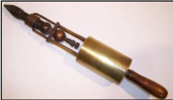
Frank J. Mann Self-Heated Soldering Iron Photo by Charles Smith
