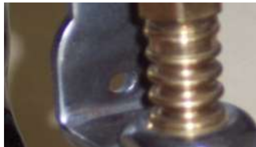
Z&W Handle Bracket w/ Hole for Heat Shield Photo by Ron Carr
