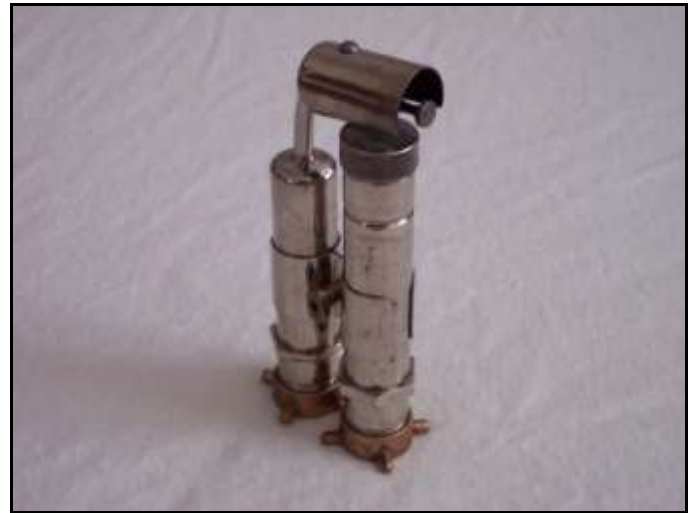
Otto Bernz model no. 13 Self-Blowing Alcohol Torch Wooden handle missing...burner cap in place. Photo by Ron Carr
