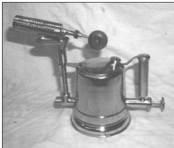
A refinished Doane & Wellington blow torch by Lloyd Patented September 3, 1882
