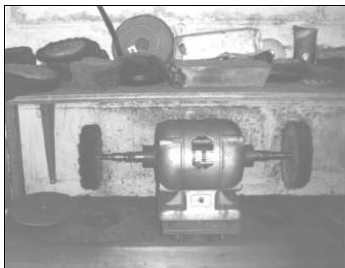
Lloyd's second motor with cotton wheels on each end
