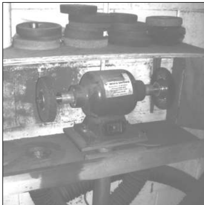
One of Lloyd's motors with a wire brush on one end and a 3M Scotch Brite wheel on the opposite side.
