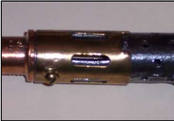
Manifold device (or shutter) on an Emmelmann Co. Blow Torch
