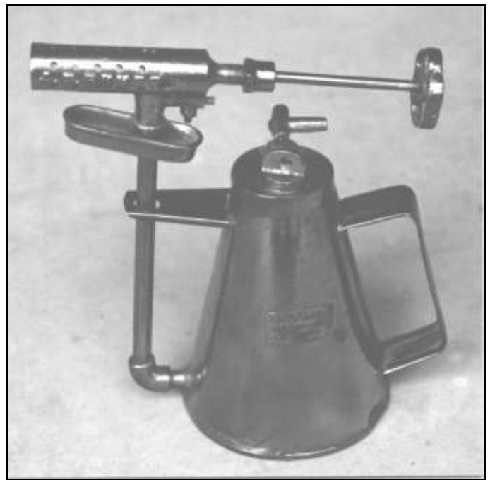
John P. Rumpf Co. blow torch, circa late 1800's Photo by Charles Smith
