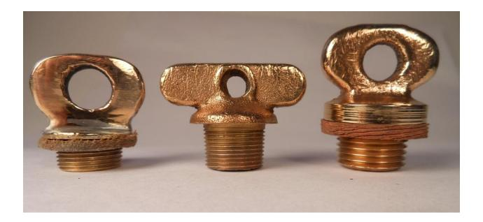
None of the above plugs are interchangeable with each other. The Frasse plug is unique and a standard 16 plug will not thread into the filler hole of the Frasse upper casting. The upper casting of the Frasse differs in other ways from standard White and even Turner-White model 16 torches.
