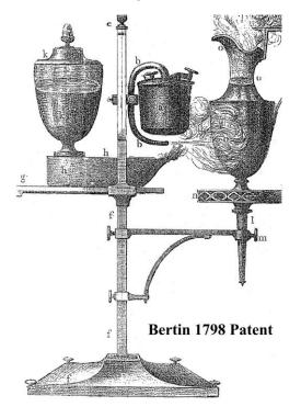
Bertin placed a sealed container of liquid above the flame from a lamp, and used the pressure generated by expansion of vapor in the upper container to create a blast via a pipe with a fine jet pointed though the flame below. Blowtorches based on Bertin's principle would continue in use for more than a hundred years.
