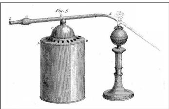
prevents air from exiting that end, and the pressure of the displaced water maintains a constant flow of air from the jet toward the flame.
