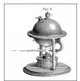
The blowpipe is connected via a hole in its side, to the top of a canister, upon which it sits. The canister is open at the bottom and is suspended inside a larger container, which is partially filled with water. When air is blown into the blowpipe, the greater part enters the first canister, displacing some of the water into the annular space between the two cylinders. A valve in the blowpipe mouthpiece
